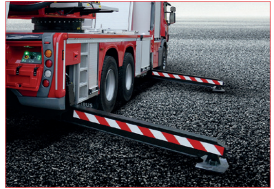
XLL VARIO jacking system
